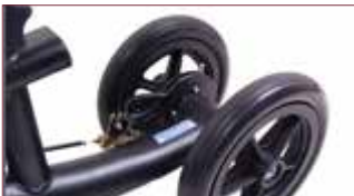
Superior treaded tires and drum-braking system
